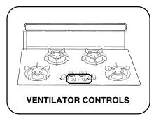
The ventilator is a 500 CFM exhaust system that can be hidden away when not in use. It has a variable speed blower. The amount of drawing power can be adjusted to the cooking job; HI exhaust for frying, LO for light simmering, or anywhere in between.
